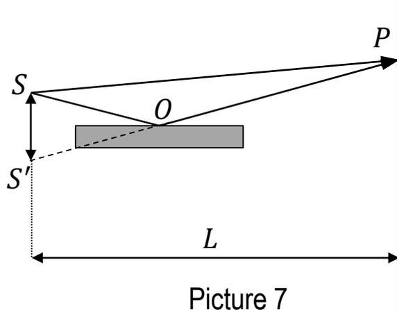
Another simple, yet ingenious, arrangement for producing an interference pattern with a single light source is known as *Lloyd's mirror*. A point source of light is placed at point S, close to a mirror, as illustrated in picture 7.
