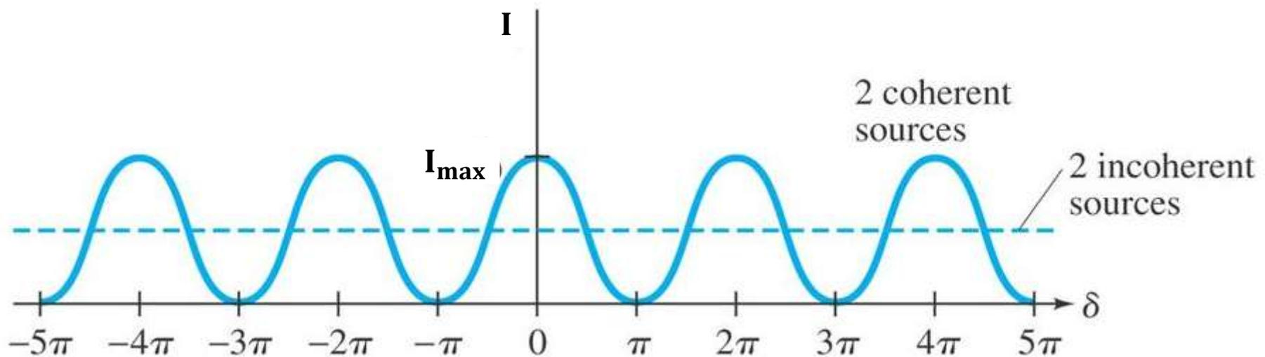
Picture 4: Distribution of the intensity as function of phase difference  $\Delta\varphi$
